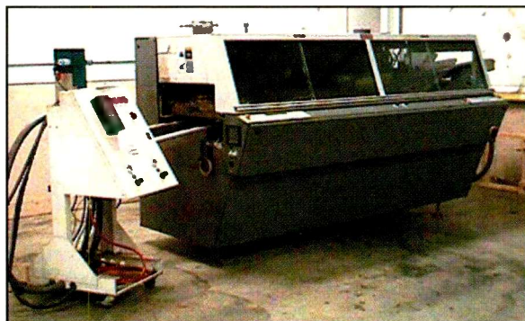
This is how circuitry is soldered today. No more soldering irons or people working on assembly lines. Instead the circuit boards are passed through a machine where all soldering takes place through automated processes. Fewer people are involved, there are fewer mistakes, and the savings are passed on to you.
