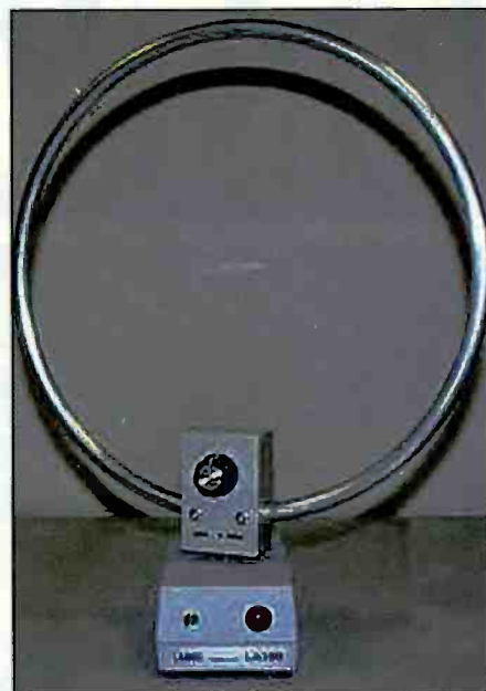
AOR makes this active shortwave loop antenna, which covers 3 to 30 MHz.
