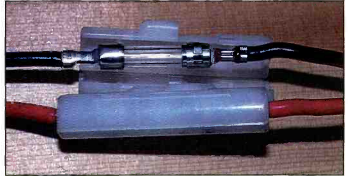
A two-way radio suffering from "brown-out" may have an open black lead fuse.
