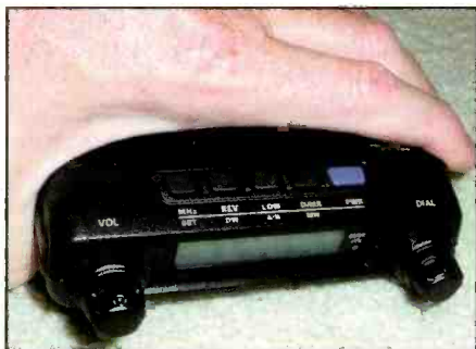
The 50-watt FT-1500M transceiver just about fits into the palm of your hand.
